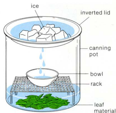
FIGURE 24.16 A simple apparatus for distilling mint oil at home.
